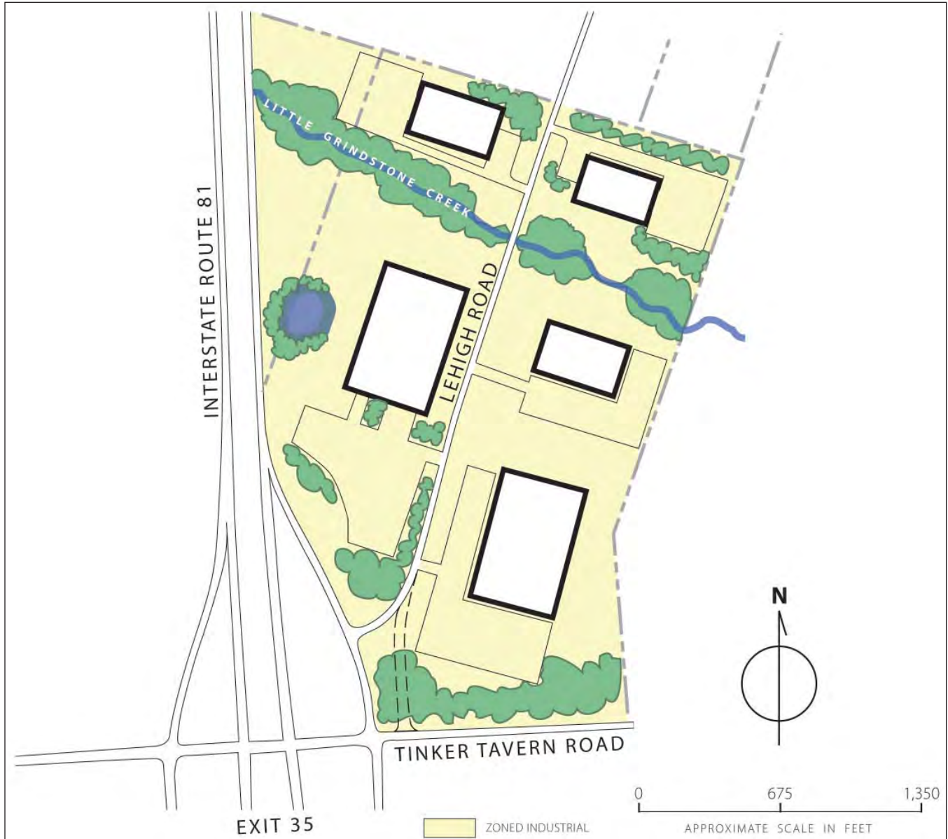
Figure 16. (above) A conceptual pre-development plan for a Tinker Tavern Exit Industrial Use area illustrates space carefully organized for maximum potential development that could be phased in over time. Parking is organized efficiently and screened from view to protect the surrounding rural character of the area. In addition, natural resources such as Little Grindstone Creek are protected with dense vegetated buffers and visual breaks where views from adjacent office areas can be enjoyed. Note dashed line indicating a change in realignment of Lehigh Rd. from its existing location on the interstate on ramp, to Tinker Tavern Rd.
